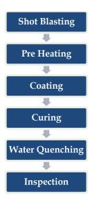
Stage 1: Surface preparation - Airless (Wheel Blast) Shot Blasting Process
